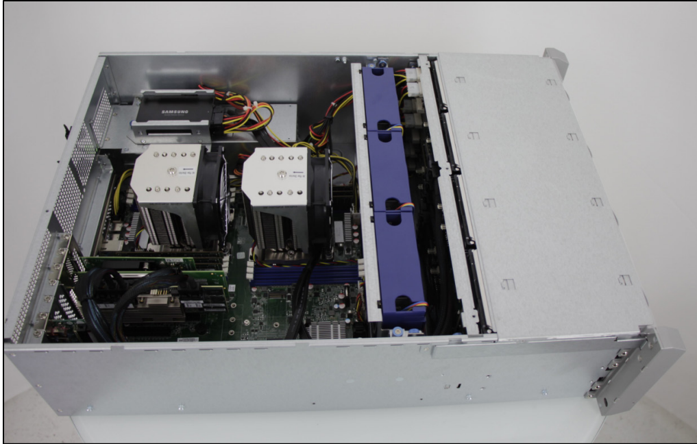
Figure 1. weather.niu.edu server with the protective top case removed. 2x CPUs, RAM, and SSD drives are easily visible.
